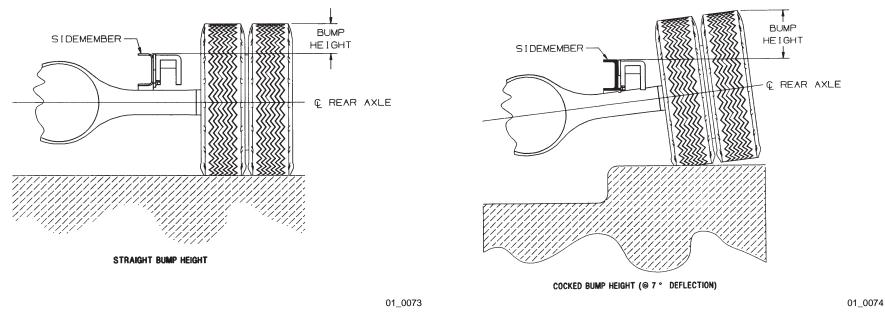
Wheel Axis to bottom of frame in straight bump position. Refer to tabulated data.
