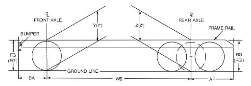
FIRST WE MUST DETERMINE THE RAKE OF THE FRAME (I.E., THE SLOPE OF THE FRAME FROM FRONT END TO REAR END). IF THE FRONT END OF THE FRAME IS HIGHER THAN THE REAR END (I.E., > OR Y'> ') THEN THE TRUCK IS SAID TO HAVE A NEGATIVE RAKE. IN THIS SITUATION, THE EQUATIONS FOR DETERMINING THE FRAME HEIGHT AT THE RAIL ENDS ARE:
