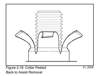
The fastener will come free when sufficient collar material has been pulled away (Figure 2.19).
