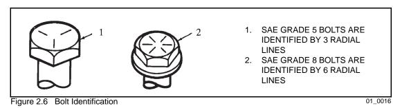
These bolts, 0.5 inch (13 mm) diameter flange head type, should be tightened to 110 to 120 ft-lbs. (149 to 163 Nm) based on new bolts and nuts lubricated with engine oil. Whenever possible, hold the bolt and tighten the nut.
