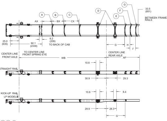
A(B)(C) SINGLE STAMPED CROSSMEMBER MOUNTED WITH FLAT FLANGE UP AND WEB FORWARD
