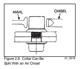
CAUTION: The HP 8 fastener is not intended for re-use. To do so can result in damage to the vehicle frame or components attached to the frame.
