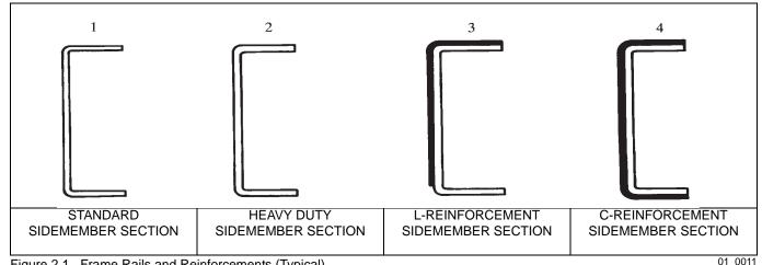
Figure 2.1 Frame Rails and Reinforcements (Typical)
