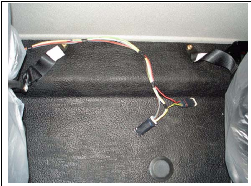
7-Way and 3-Way Connectors for 08HAU (Inside Cab)
