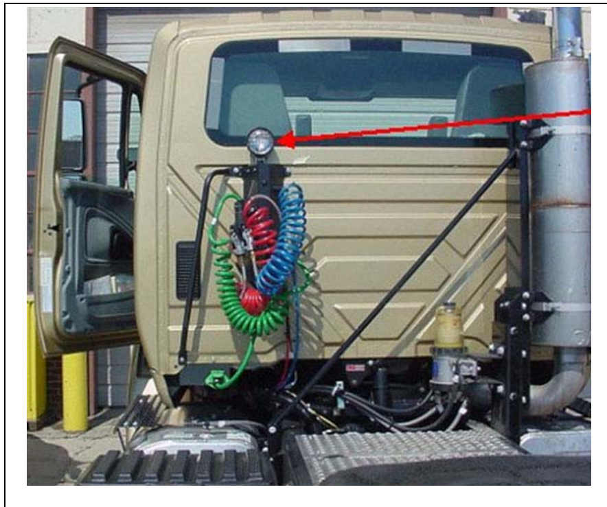
Arrow Indicates Location of Work Light (Tractor) f_063
