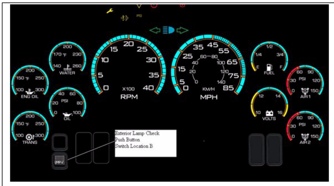
Push Button Switch Located Below the Instrument Cluster (595AZY)
