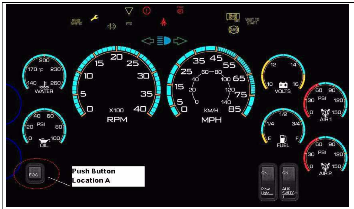
Fog Light Switch Located Under the Instrument Cluster
