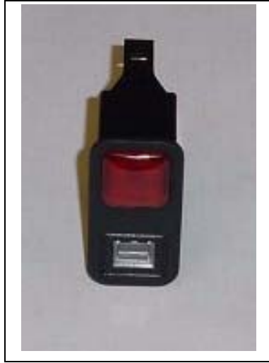
Indicator Light Included f_120 Location: Center Multiplex Panel in Dash Switch
