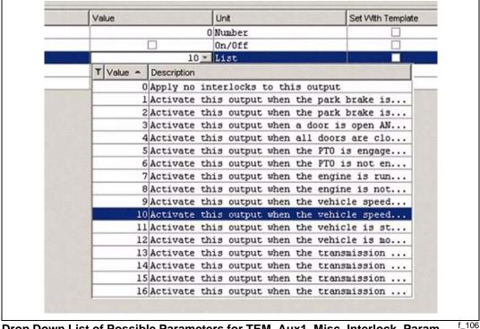
Drop Down List of Possible Parameters for TEM\_Aux1\_Misc\_Interlock\_Param <sup>f\_10</sup>
