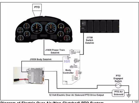
Diagram of Electric Over Air (Non-Clutched) PTO System
