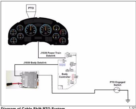
**Diagram of Cable Shift PTO System**
