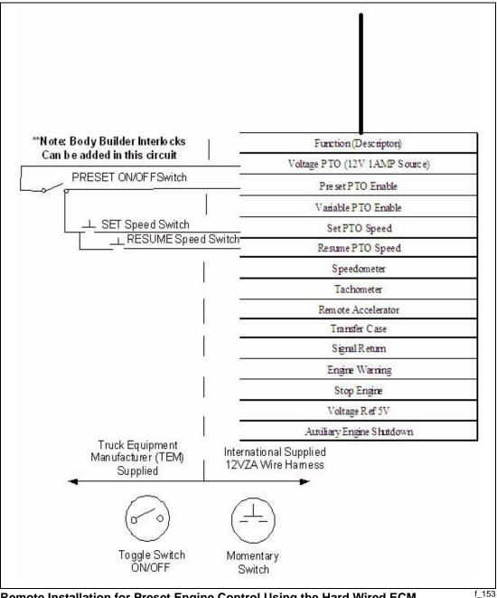
Remote Installation for Preset Engine Control Using the Hard Wired ECM Inputs
