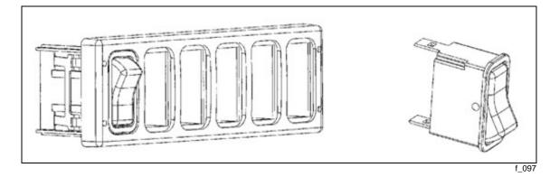
Most switches are rocker actuators that do not require hard wiring. See the Switch Actuators for Multiplex Systems Table below. The switches are used in switch pack modules (6 or 12 switches) that connect to the multiplex system through the switch housing cable harnesses. Push button switches for the cluster are also available. See Push Buttons Table below.
