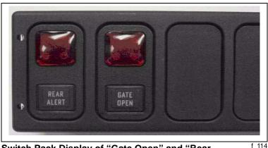
Switch Pack Display of "Gate Open" and "Rear Alert" Indicator Lights
