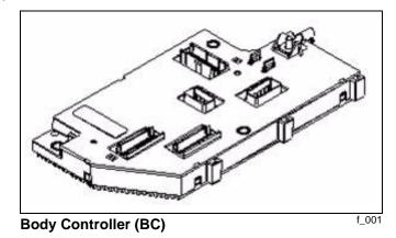
The BC communicates with the switch packs on the switch datalink, controllers from other features on the power train datalink, and RPMs (remote power modules) and the RESCM (remote engine speed control module) on the Body Builder datalink. It also receives input from various sensors and hard wire inputs throughout the truck. The BC converts these inputs, in accordance with the programmed "rules," into data to be transmitted on the datalinks.
