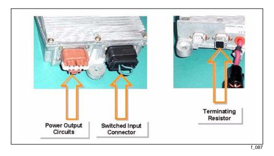
When more than one Remote Power Module (RPM) is installed, the Data Link wire harness must be daisy-chained using the scheme diagrammed in the figure below. Connect the 6 pin Data Link Harness (J1939) from the first RPM to either data link connector of the second. Continue connecting the data link jumper
