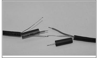
Put Heat Shrink Tube Over Each Wire
