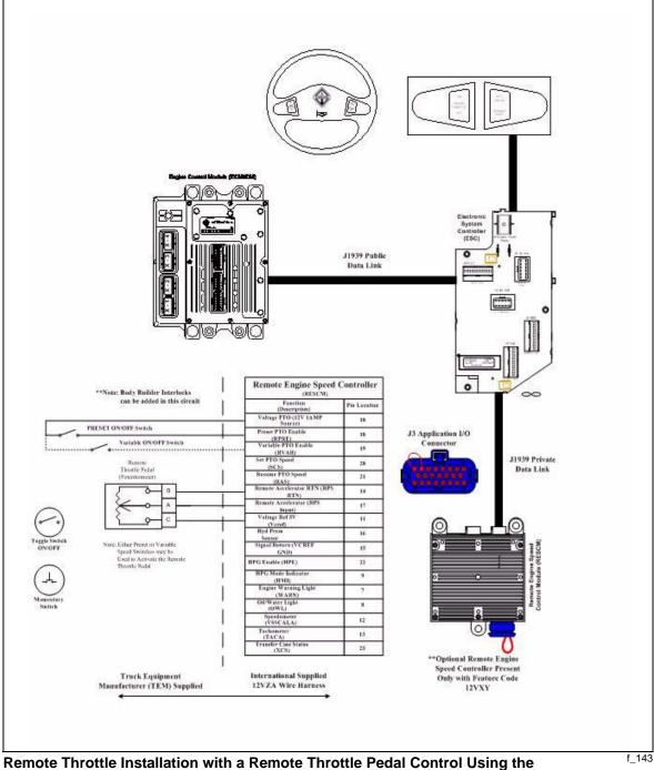
Remote Engine Speed Controller (RESCM)
