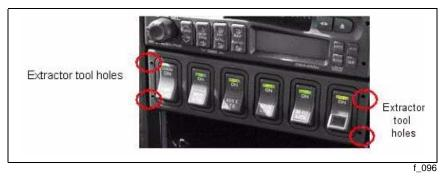
To remove individual switches or blanks from a switch pack, squeeze the locking tabs on the rear of the switch or blank (top and bottom) and push it from the housing.
