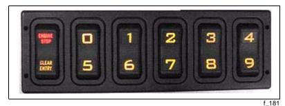
The red ENGINE STOP indicator portion of the ENGINE STOP/CLEAR ENTRY switch flashes to alert the driver that the theft deterrent code must be entered (within the preprogrammed time delay or the engine will shut down). The momentary CLEAR ENTRY position is pressed whenever the driver needs to clear a failed code so that the correct code can be re-entered.
