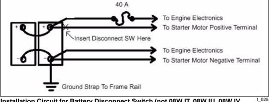
Installation Circuit for Battery Disconnect Switch (not 08WJT, 08WJU, 08WJV or 08WJW)
