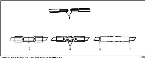
**Crimp and Seal Splice Sleeve Installation**
