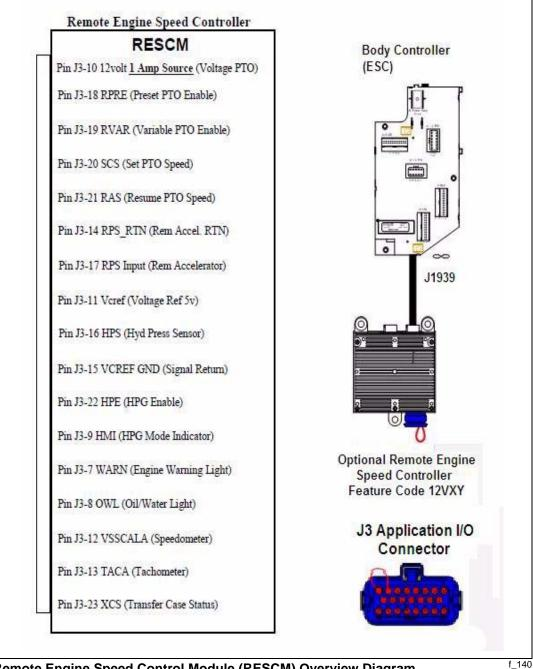
Remote Engine Speed Control Module (RESCM) Overview Diagram
