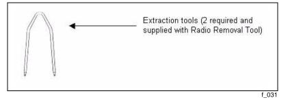
Insert the extraction tools (2) into the two holes on either side of a switch pack housing until the locking tabs are fully depressed. The switch pack can then be removed from the panel and the extraction tools removed.
