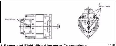
3-Phase and Field Wire Alternator Connections
