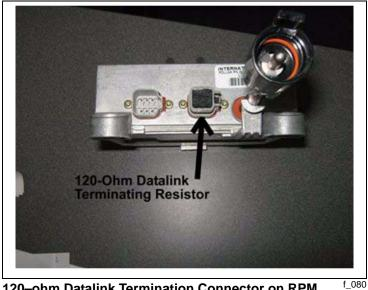
120-ohm Datalink Termination Connector on RPM
