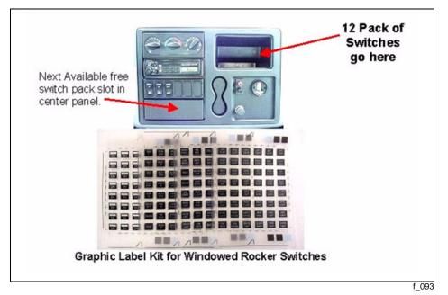
If an additional switch pack is being installed, it is connected to the multiplex system by "daisy chaining" its connectors to the existing switch pack (or to the cab harness if no switch pack is currently installed). It is important to connect the switch packs in the correct order. Connecting the switch packs together and to the cab harness in the wrong order will cause switch pack addressing problems.
