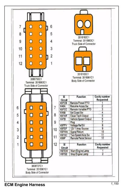
If the Engine Harness is not provided, the following diagrams show how to hard-wire this feature.
