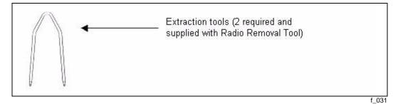
Insert the extraction tools (2) into the two holes on either side of a switch pack housing until the locking tabs are fully depressed. The switch pack can then be removed from the panel and the extraction tools removed.
