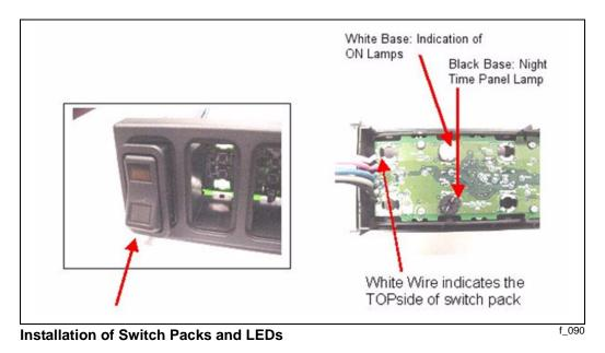
To install a switch in the switch pack housing, insert the switch in the proper slot and push in until the switch locking tabs are fully engaged (switches are keyed and cannot be installed upside down).
