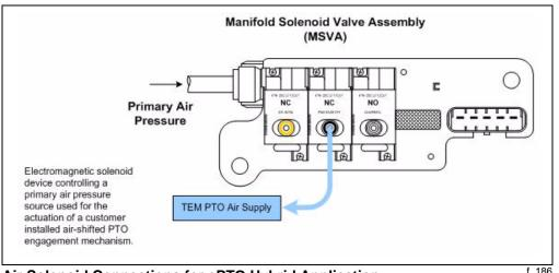
Air Solenoid Connections for ePTO Hybrid Application
