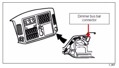
To connect to this circuit, remove the lock from the wire side of the bus bar connector and insert the added wire with terminal (terminal part number 1661208C1) on an unused connection point.
