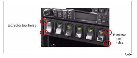
To remove individual switches or blanks from a switch pack, squeeze the locking tabs on the rear of the switch or blank (top and bottom) and push it from the housing.
