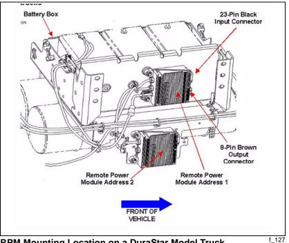
RPM Mounting Location on a DuraStar Model Truck
