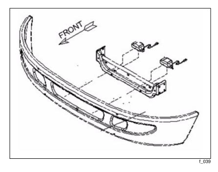
Thin fog lamps must be used if mounted in the bumper opening of the 3200, 4200, 4300 and 4400 models.
