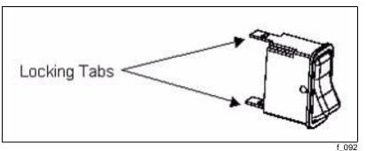
To install a switch in the switch pack housing, insert the switch in the proper slot, and push in until the switch locking tabs are fully engaged (switches are keyed and cannot be installed upside down).
