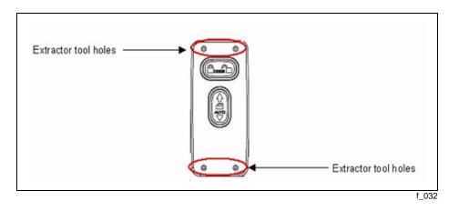
To install the new replacement pod, connect the appropriate connectors and push the pod in until the locking tabs are fully engaged.
