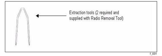
Insert the extraction tools (2) into the two holes on either side of the pod housing until the locking tabs are fully depressed. The pod can then be removed from the door panel and the extraction tools removed.
