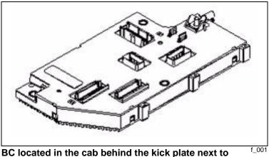
BC located in the cab behind the kick plate next to the driver's left foot
