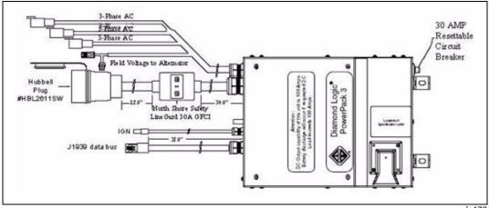
PowerPack 3 Inverter/Regulator Component Detail
