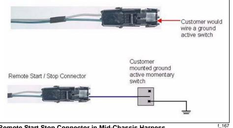
**Remote Start Stop Connector in Mid-Chassis Harness**
