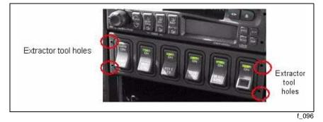
To remove individual switches or blanks from a switch pack, squeeze the locking tabs on the rear of the switch or blank (top and bottom) and push it from the housing.
