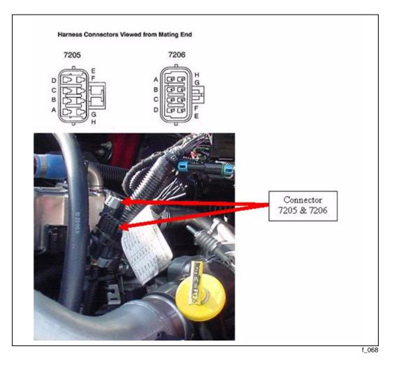
To use these connectors, remove cavity plugs and use the following:
