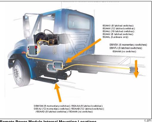
**Remote Power Module Internal Mounting Locations**
