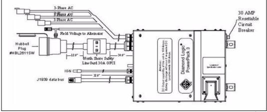
PowerPack 3 Inverter/Regulator Component Detail
