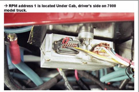
**RPM Mounting Location on a WorkStar Model Truck**
