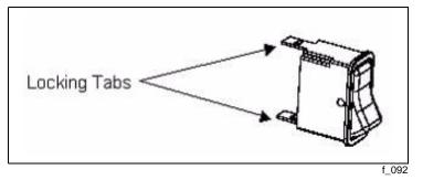
To install a switch in the switch pack housing, insert the switch in the proper slot, and push in until the switch locking tabs are fully engaged (switches are keyed and cannot be installed upside down).
