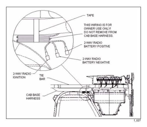
08REA and 08RGA provide radio power and GND directly from the battery to minimize electrical noise on the line.
