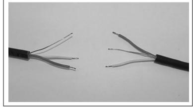
**Re-Twist Any Loose Wires**
