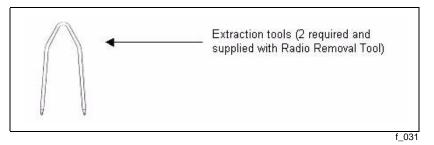
Insert the extraction tools (2) into the two holes on either side of a switch pack housing until the locking tabs are fully depressed. The switch pack can then be removed from the panel and the extraction tools removed.
